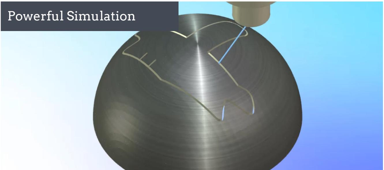
CIMWorks WireEDM also features powerful simulation powered by Predator Virtual CNC, allowing you to check for accurate toolpath, collisions, and machining order all before taking code to the machine. Simulate with WIP models, and streamline your design and planning process.
