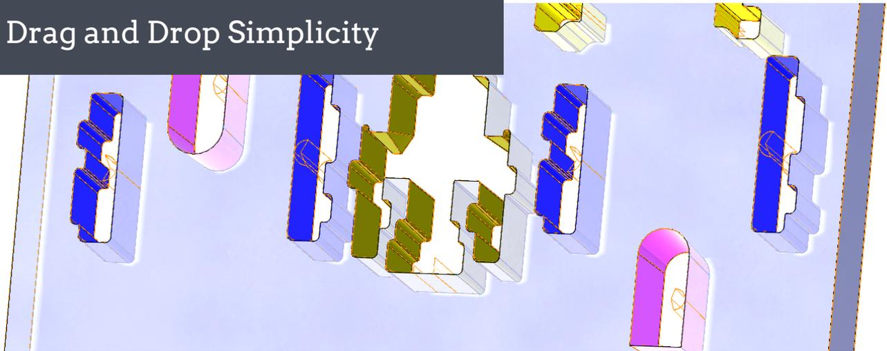
Our color-coded and decal-defined strategies allow you to customize your machining processes and user technology. Apply the corresponding color and CIMWorks WireEDM will identify the strategy or surface finish and apply it to the colored features, minimizing time and error. Drag a decal on to the desired face and the system will identify approach strategy and the use of tabs and stop points, allowing for unprecedented control during feature recognition.
