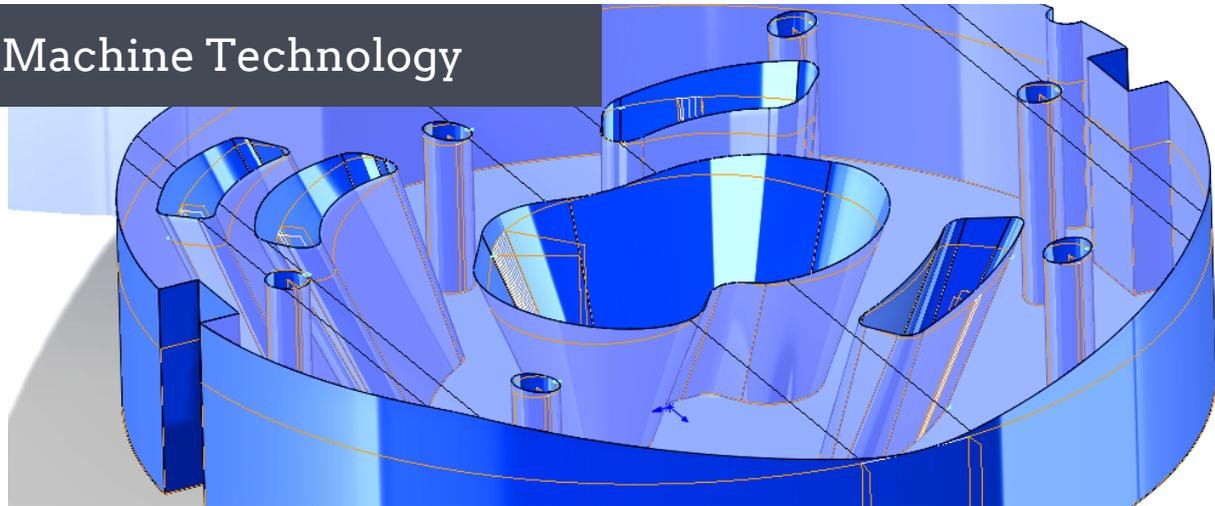
Our automatic feature recognition has evolved to 2 Axis, 2 Axis w/taper and 4 Axis synchronized and un-synchronized from a solid model. The requirement of several 2d sketches to define top and bottom cuts is virtually eliminated. Even the requirement for a planar surface is a thing of the past. Plus, the ability to automatically program from a 2d wire frame still exists. This gives you control when you need it and saves time when you don't.
